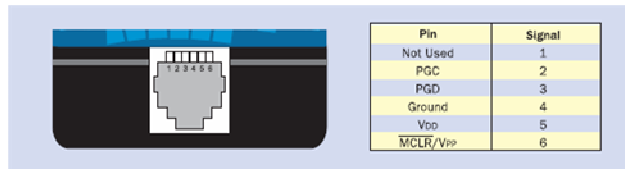
Figure 5 - ICD2 RJ-12 Pinout
