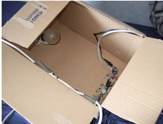
Figure 8 – Test-bed, with heat source off
